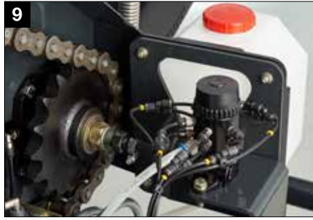
9 BEKA-MAX continuous chain oiling system
