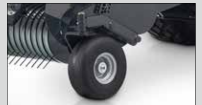
Pivoting semi-pneumatic pick-up guide wheels
