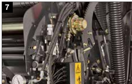
Proportional valve for in-cab density control
