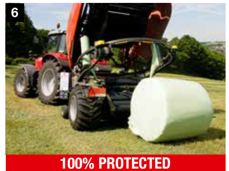
6 100% PROTECTED Once the bale is completely protected, it is gently unloaded by the machine. Thanks to the design of the bale chamber, the drop height is kept as low as possible. Optionally, the machine can be equipped with a bale turner, to turn the bale onto its flat end
