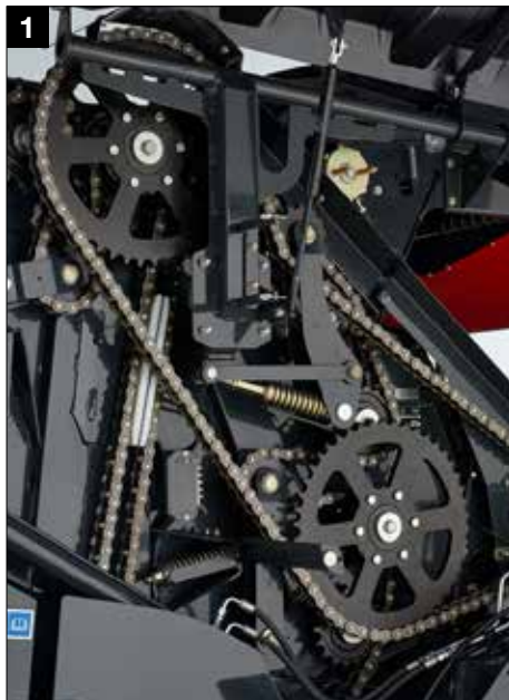
Robust driveline with high quality IWIS chains
