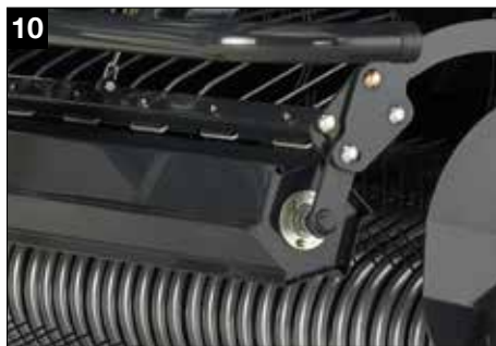
Heavy crop roller with a windguard (Ø 217 mm)
