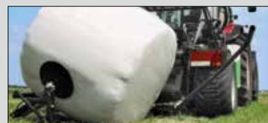
Bale turner, unloading the bale on its flat end
