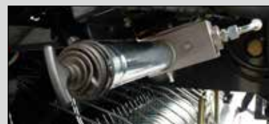
BEKA-MAX automatic bearing greasing system
