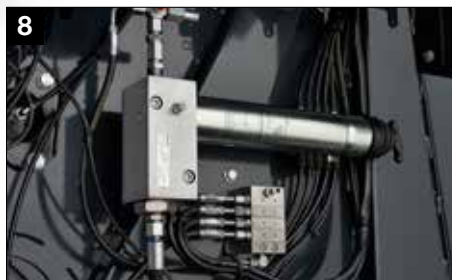
8 Standard automatic greasing system for roller bearings
