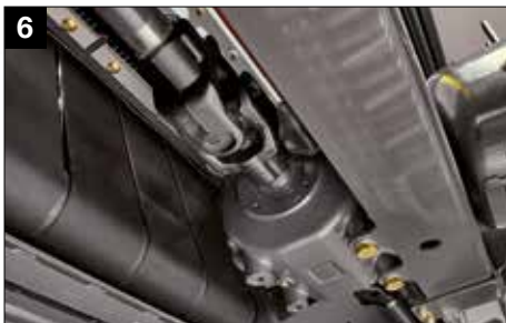
Heavy duty cross joints in the drive axles
