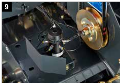
BEKA-MAX continuous chain oiling system
