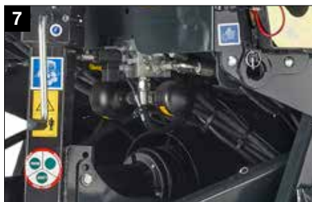
7 Proportional valve for in-cab density control as standard
