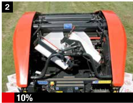
2 10% Once the film is being applied to the bale, the two film reels tilt to a horizontal position. Using of two reels ensures the film is at full width after about half a turn of the bale
