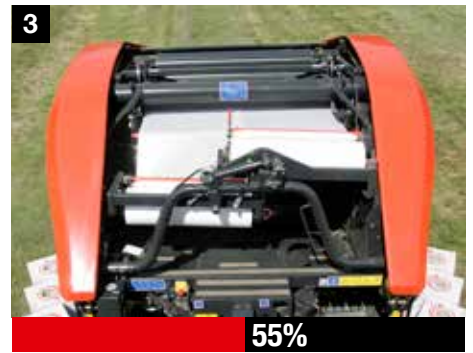
3 55% The number of layers can be conveniently set via the ISOBUS terminal. The high pre-stretch ratio of the film results in 30% film cost savings and even more so during film binding with pre-stretched film
