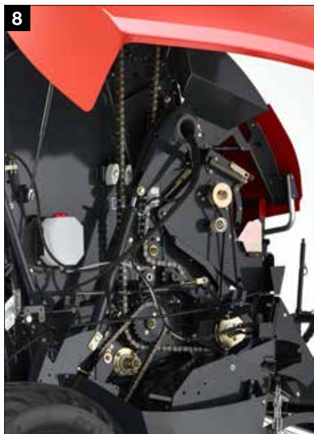
Robust driveline with high quality IWIS chains + 1 1/4" 20BH primary driveline with chrome hardened pins
