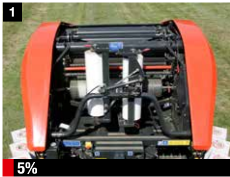
1 5% The film binding cycle starts with the film reels in the upright position. This ensures that the binding material is applied in 2 strands directly and firmly onto the bale surface
