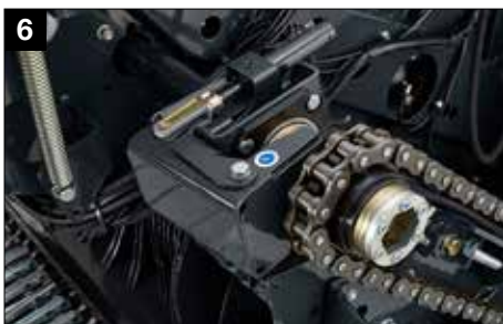
6 Standard hydraulic rotor disengagement
