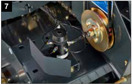
BEKA-MAX continuous chain oiling system
