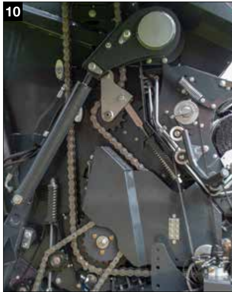
10 Robust driveline with wear-resistant and oversized chains
