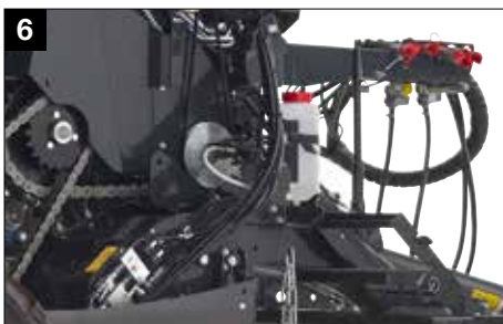
6 BEKA-MAX continuous chain oiling system
