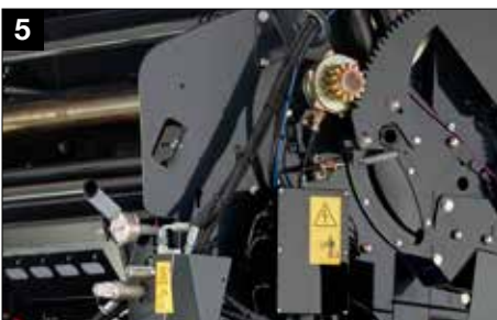
Proportional valve for in-cab density control
