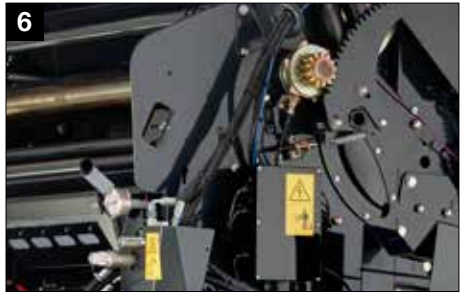
Proportional valve for in-cab density control
