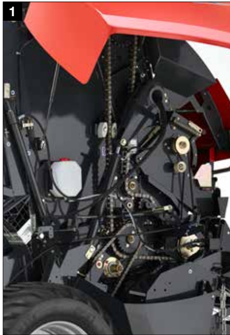
Robust driveline with high-quality IWIS chains
