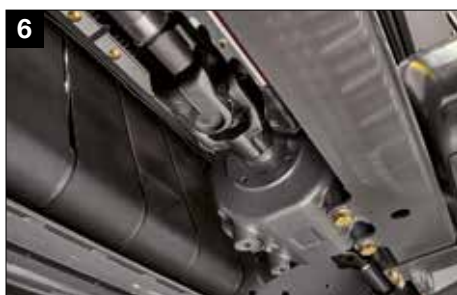
Heavy-duty cross joints in the drive axles
