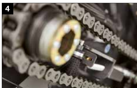
4 Sturdy and wide oil brushes on the chains ensure perfect lubrication
