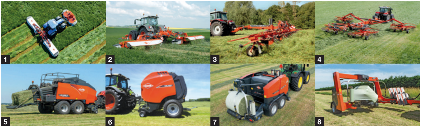
1. Triple gang mowers - 2. Triple gang mower conditioners - 3. Large width tedder - 4. 4-rotor rake - 5. High density baler - 6. Round baler - 7. Fixed chamber baler-wrapper combination - 8. Wrapper.
