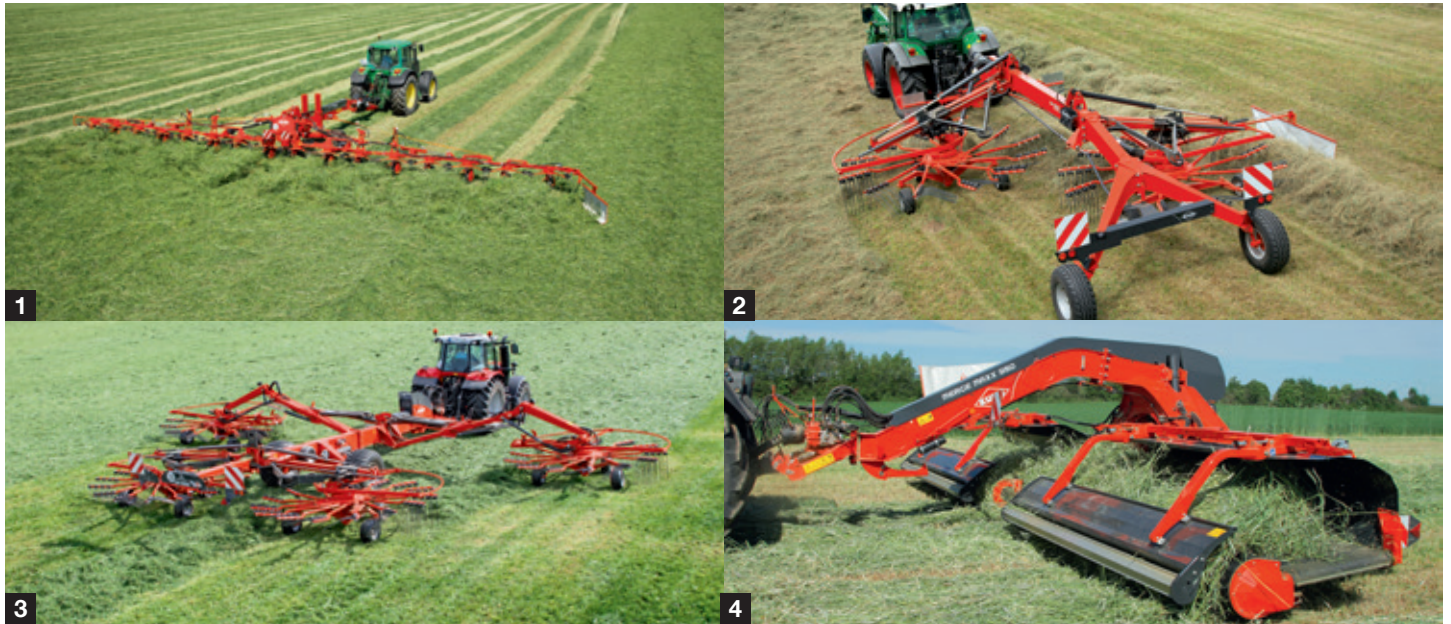
1. Gyrotedders up to 17 m 2. Twin-rotor Gyrorakes 3. Four-rotor Gyrorakes 4. Belt mergers up to 13 m
