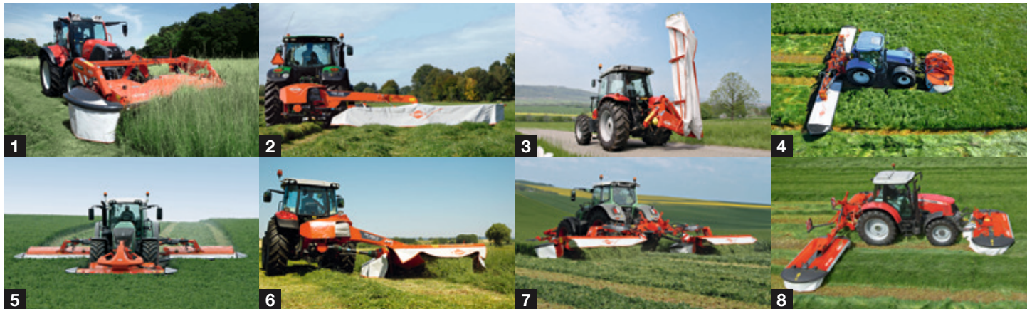
1. Front disc mowers 2. Horizontal fold disc mowers 3. Vertical fold disc mowers 4. Triple gang disc mowers 5. Front disc mower conditioners 6. Mounted disc mower conditioners 7. Triple gang mower conditioners 8. Drum mowers
