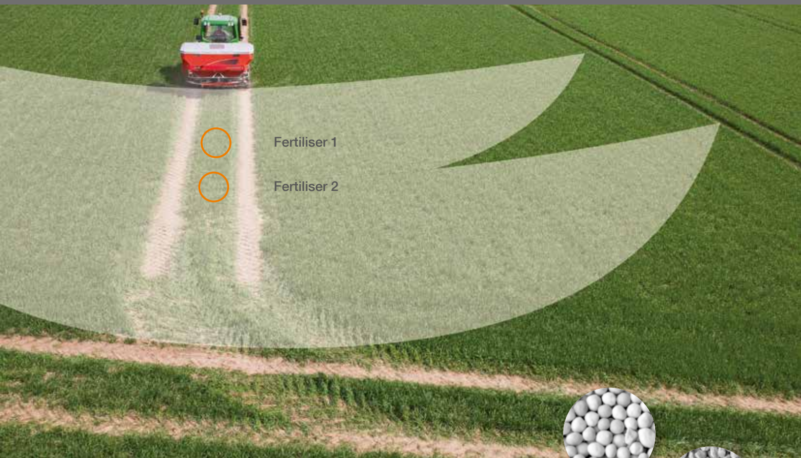
Ideal switch points for different fertiliser types
